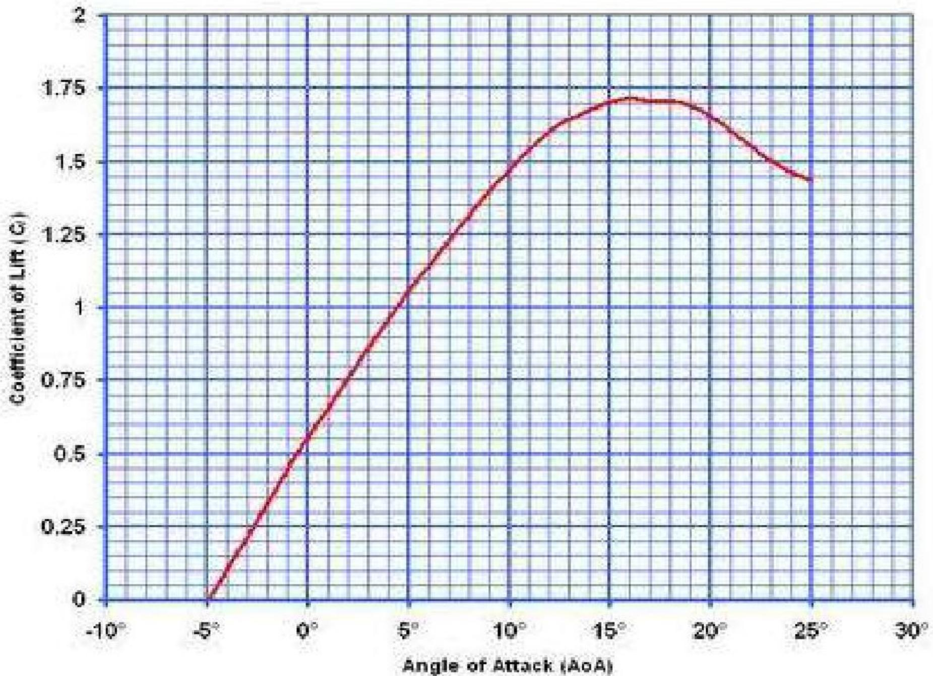
The graph below shows how lift and drag changes with the angle of attack for a typical wing design.
